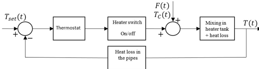
Figure 4: General control loop scheme for water heater system
