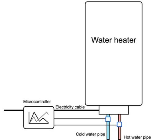
Figure 1: Schematic view of the heater system
